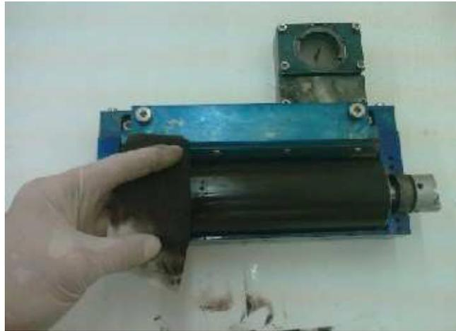
If the anilox roll appears significantly free of silver after cleaning with soapy water than it can be used without proceeding to the following steps. However, if there appears to be silver residue or the cells are entirely clogged with silver as pictured below then the following steps can be used to remove all remaining silver residue.
