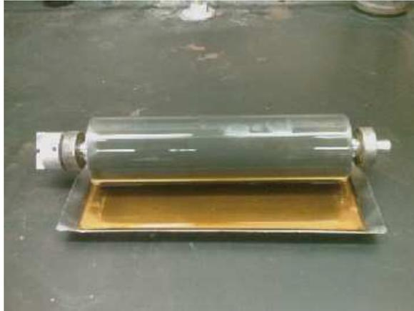
**Step 3:** Wipe down excess ferric nitrate solution with a rag and dispose of rags and ferric nitrate solution properly.
