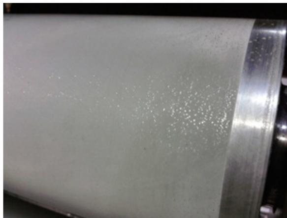
**Step 2:** Wipe down the anilox with a dry rag to remove residual soap. Submerge the outer surface of the anilox roll in a shallow pan with ferric nitrate solution. Rotate to evenly coat anilox surface continuously for 10-15 minutes. Alternatively the ferric nitrate solution can applied using a pipette or sponge while being scrubbed with a rag, sponge, or a wire brush. ***Ferric nitrate is corrosive, and should not come into contact with the skin or eyes.***
