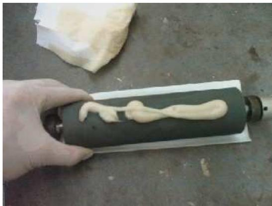
Using a clean damp rag/towel spread the Ceramclean II over the roll surface in a circular motion and agitate with a wire brush appropriate to the type of anilox roll. Rinse surface with clean water to make certain all the cleaner is removed from the surface of the roll.
