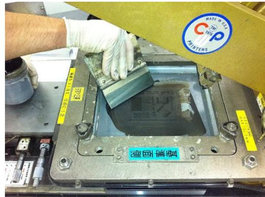
**Step 1:** Keep the screen flooded with ink until ready to clean. Scrape or squeegee off the bulk of the ink from screen thereby leaving the open mesh areas filled with wet ink. **Immediately proceed to Step 2!**
