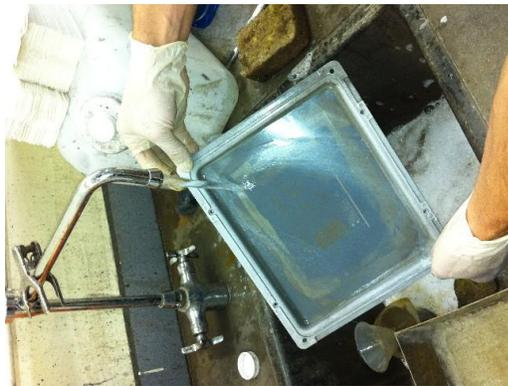
**Step 4:** Rinse with water, dry frame with towel, air dry mesh before reuse.
