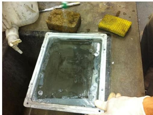
**Step 2:** Wet the top and bottom surface of screen mesh with soapy water solution.
